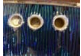
This method produced some chipping of the glass and removal of the backing material.
