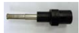
5/8 - 11 adaptor with drill bit attached
